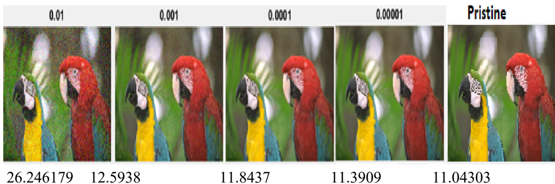
Figure 13: Pristine and noisy versions of the same image taken under 4 different variance conditions and its corresponding 'Quality Score' values
